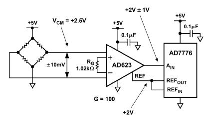
Figure 2-29: Single-supply data acquisition system
