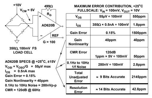
Figure 2-24: AD620B bridge amplifier DC error budget
