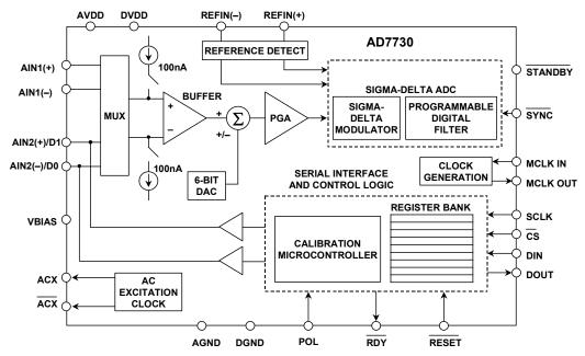
Figure 2-46: AD7730 sigma-delta measurement ADC with on-chip PGA
