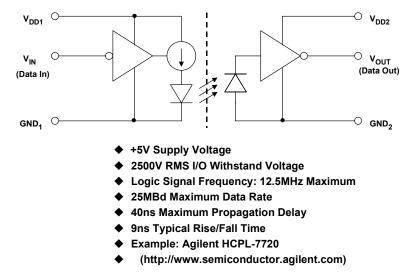
Figure 2-54: Digital isolation using LED / photodiode optocouplers
