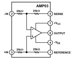
Figure 2-3: AMP03 precision difference amplifier
