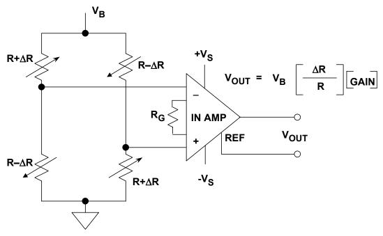
Figure 2-28: Generalized bridge amplifier using an in-amp
