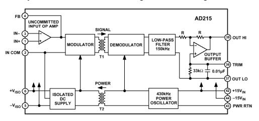
Figure 2-51: AD215 120kHz low distortion 2-port isolation amplifier
