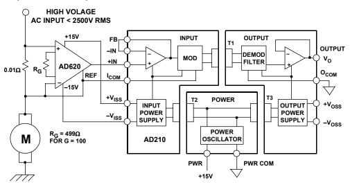
Figure 2-50: Motor control current sensing
