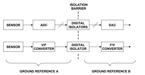
Figure 2-57: Practical application of digital isolation in data acquisition systems
