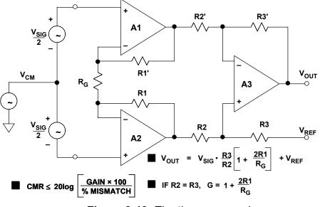
Figure 2-12: The three op amp in-amp
