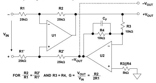
Figure 2-6: Balanced difference amplifier using push-pull feedback path
