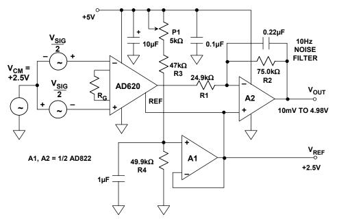
Figure 2-15: A precision single-supply composite in-amp with rail-to-rail output
