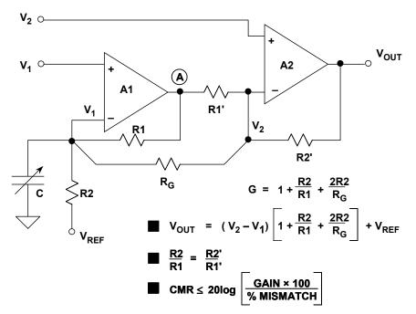
Figure 2-7: The two op amp instrumentation amplifier
