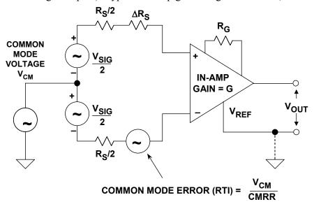
Figure 2-1: The generic instrumentation amplifier (in-amp)
