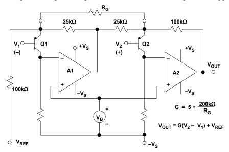
Figure 2-10: The AD627in-amp architecture
