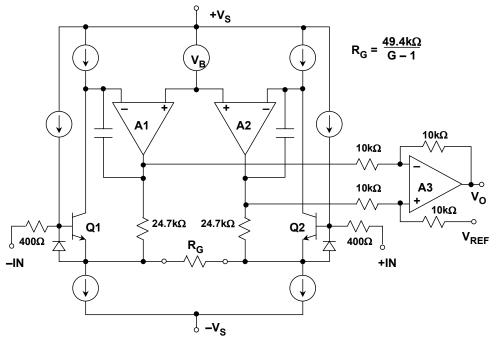
Figure 2-13: The AD620 in-amp simplified schematic
