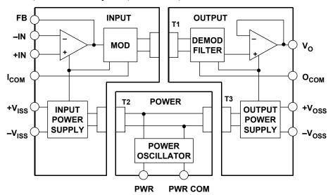
Figure 2-48: AD210 3-port isolation amplifier
