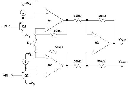
Figure 2-17: AD623 single-supply in-amp architecture
