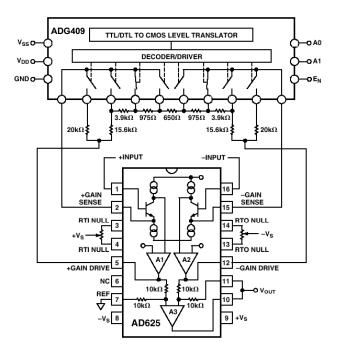
Figure 2-43: A software programmable gain amplifier
