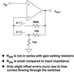
Figure 2-36: Alternate PGA configuration minimizes the effects of R<sub>ON</sub>
