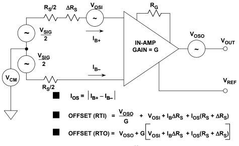
Figure 2-19: In-amp offset voltage model
